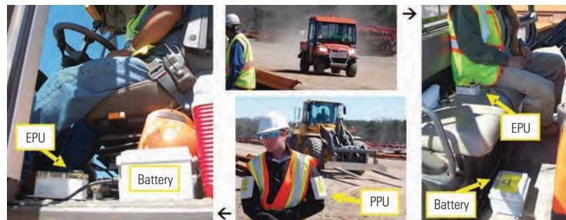
**2. Double safe.** Alerts are sent to workers on foot and equipment operators inside the cabin when a set proximity is reached. *Courtesy: CII*
