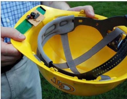
A prototype SmartHat tag attached to a hard hat
